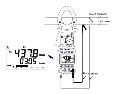
NOTE: When you turn the selector to EX-P to measure voltage or power parameter, the
