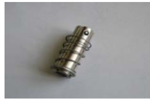
Plunger with fixed conical & cylindrical seal (Old Plunger) Photo – 6
