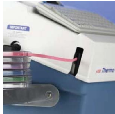
Figure 3 — Label Tape Storage Rack Installation
