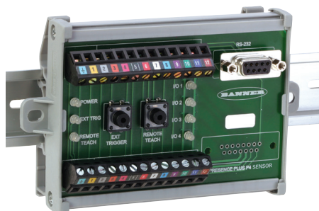
Model PPSIM..T (Terminal strip connection)
