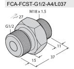
Screw-in adapter for flow sensors in the F(T)CST series for screwing into a T-piece or a welding sleeve; process connection G1/2" external thread
