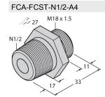
Screw-in adapter for flow sensors in the F(T)CST series for screwing into a T-piece or a welding sleeve; process connection 1/2" NPT external thread
